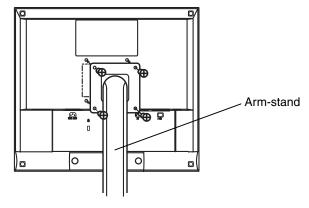
4 Mounting Screws (enclosed): M4 x 12 mm
