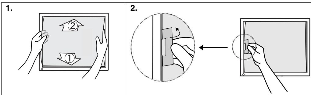
**1. Set the panel protector into the grooves of the panel frame; the lower first (1), then the upper (2).**
