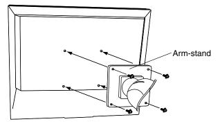
M4 Mounting Screws: M4 x 15 (mm)
