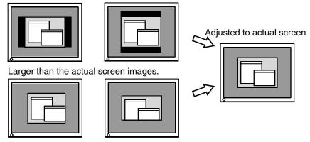
4. Adjust the output signal range (Dynamic Range) of the signal.  $\rightarrow \mathbf{\Sigma}$  Use the <Range Adjustment> (p. 50) of <Screen> menu.
