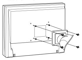
Clearance between the screw holes when attach an arm or stand: In case of 100mm x 100mm
