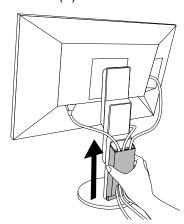
2. While holding down of (A) lightly, slide (A) upward to detach it from the stand.
